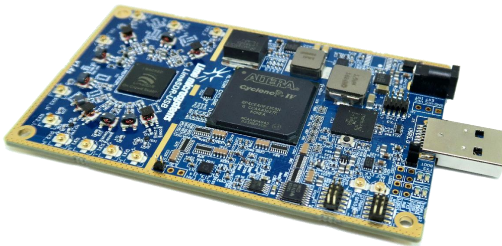
Figure 2 LimeSDR – USB type A connector board
